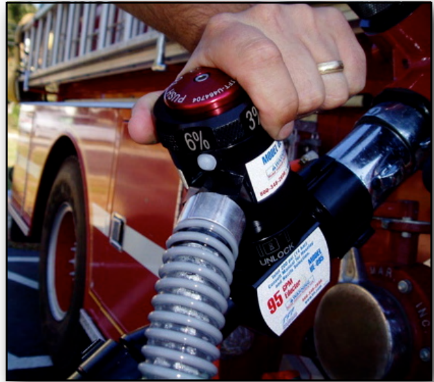
Self-Flushing eductor designed for very viscous alcohol type foams.
