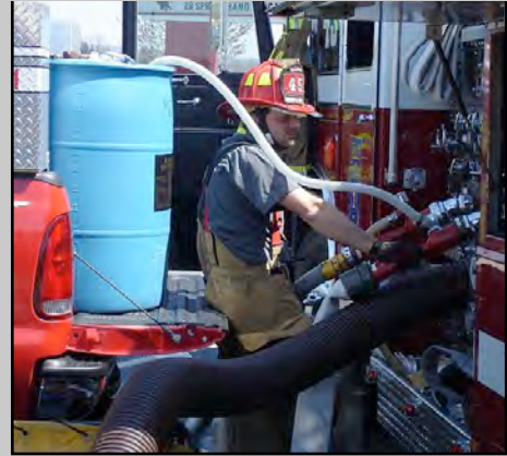
Eductor on pump discharge, not 50' down the street... Try it!
