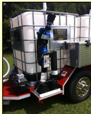
Dismounted Foam Monitor
