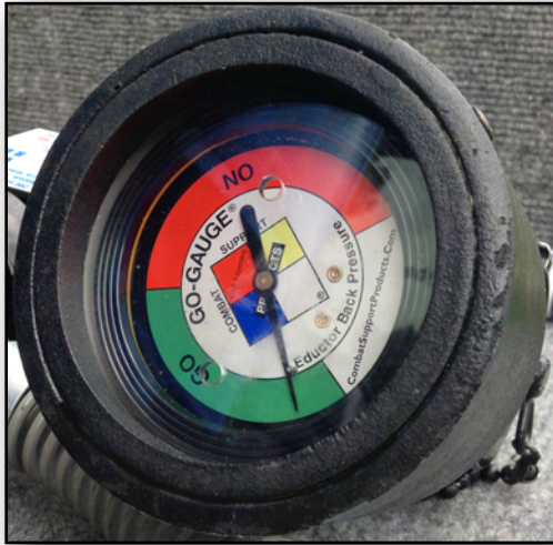
Hardened gauge enclosure with 0.25" vented Lexan cover
