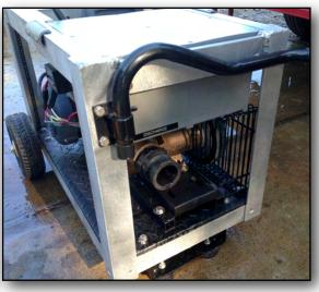
Radio controlled, wheeled unit comes with 2 -12 ft. sections 2" transfer hose and two 54" stingers. Designed for use with the most viscous AR-AFFF foam concentrates.
